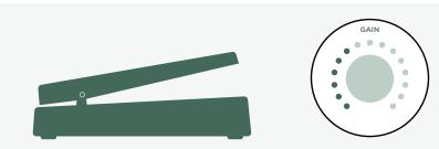
Move the pedal to toe position. Turn the **GAIN** knob and select the intended level for your Morph Sound.
