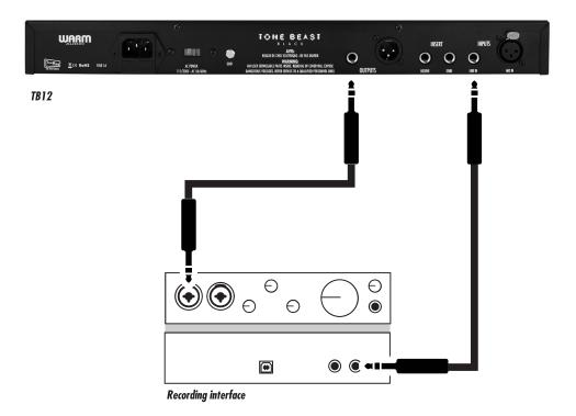
In this example, the TB12 Black is being routed as an insert into a recording device. This is useful for using the TB12 Black as an "analog plug-in" or insert for mix-down. The recording device is feeding the TB12 Black with a balanced 1/4" cable via a line output. Then, the recording device is capturing the TB12 Black via a LINE LEVEL input.
